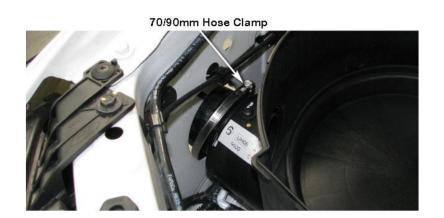
Loosely install the 90/110mm hose clamp (Item 12) onto the air entry hose (item 10).
